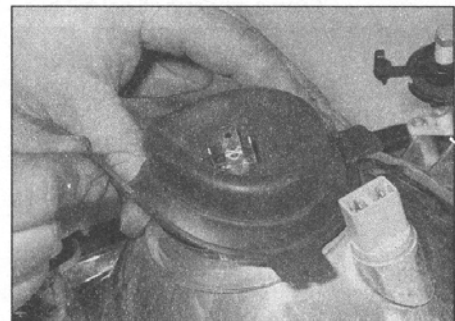
5.9a On later models, with the headlight on the bench, remove the rubber dust cover . . .
