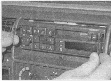
21.4a . . . then insert the removal tools and slide out the radio/cassette unit . . .
