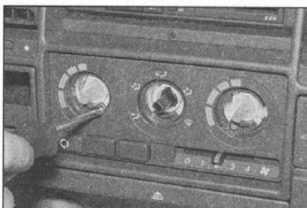
6.20 . . . then undo the retaining screws and remove the front plate from the heater control unit
