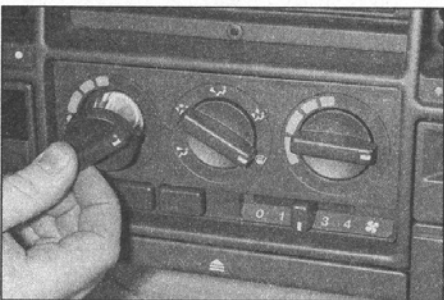
6.19 On later models, pull the control knobs off from the heater controls and the blower motor switch . . .
